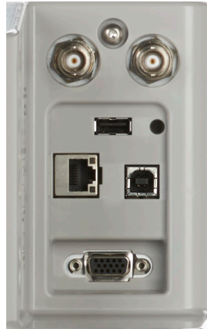
Figure 52. Connectivity section on the back panel.
