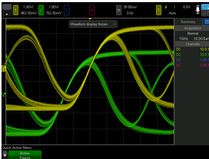
Figure 54. Quick Freeze Display preserves the persistence.
