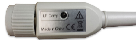
Figure 2. Low-frequency compensation adjustment (for N2840A/41A/42A/43A/53A)
