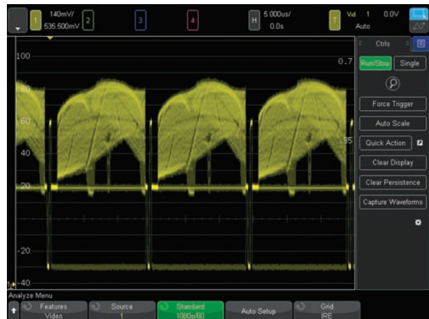
Figure 27. Triggering on 1080p HDTV signal analysis.
