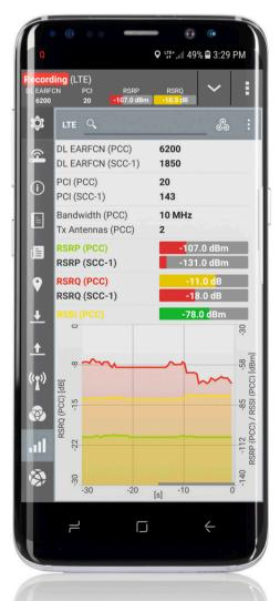
The Android based QualiPoc application running on a smartphone controls the R&S<sup>®</sup>TSMA6.
