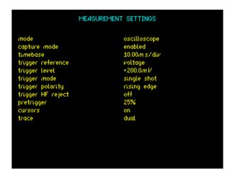
Press the enter button, the PPA display shown will now be in Oscilloscope mode.
