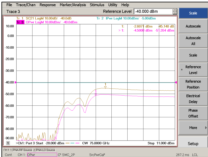
Figure 6. Swept LO at a millimeter wave frequency of 75 GHz
