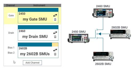
Characterize devices using up to four of Keithley's SourceMeter SMU instruments.
