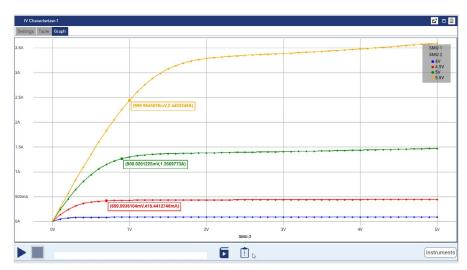
Create current vs. voltage characteristics for 2-terminal, 3-terminal, and 4-terminal devices.
