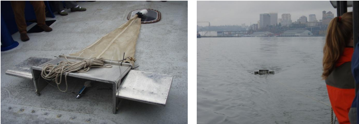
Figure 6.1 Manta trawl with flow meter (left); Manta trawl in action (right). Samples in the nets are collected in glass containers, and quantitatively transferred from the net to the container with clean drinking water (not seawater). Onboard ship, seawater microplastics samples may be treated with preservatives. To rid the sample of organic matter, a H_2O_2 step is sometimes applied. Ridding samples of organic matter is useful when visual inspection is applied to separate polymer material from other materials (Arthur et al. 2009b). Photos H.A. Leslie.
