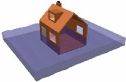
Figure 13: Wet proof construction, lets the water enter the house. Source: de Boer, 2008
