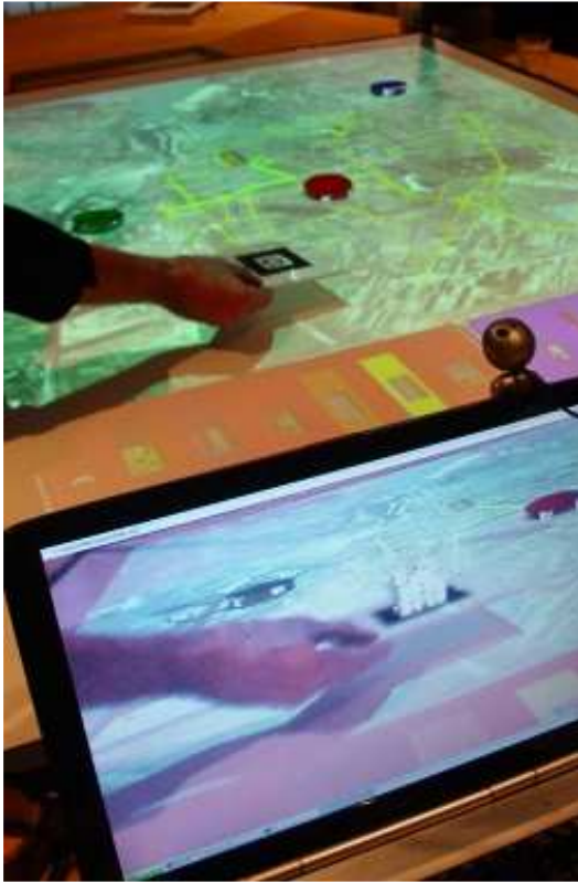
Figure 2: AR example: the tangible interface and its objects are shown on the top half of the picture. A person is holding a pattern over the table surface. In the bottom half of the image the picture captured by a simple web-cam can be seen. In the filmed image, instead of the pattern, a 3D model of an office building is visualised.
