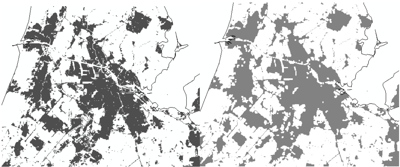
Figure 4 Built-up land use types (in dark-grey) in the year 2000 in the region around Amsterdam directly derived from the land use model (left) and after applying the Boundary Clean function (right).
