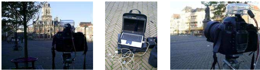
Fig. 2. Collage of the image collection on the Market square in Delft using the Nikon D100 camera mounted with digital compass on the hot shoe cover
