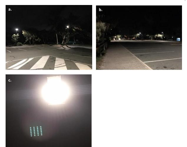
**Figure 33: Lighting in car park at Buddina Coopers Lookout/Kawana SLSC** a. looking away from the beach toward the road; b. looking south toward the SLSC and toilet block (on right of image) and c. close up of an indicative LED lighting fixture located at top of access (221) steps, taken from 2 m away. See **Figure 18** for isophote image of lighting from the nesting beach immediately adjacent to this location.
