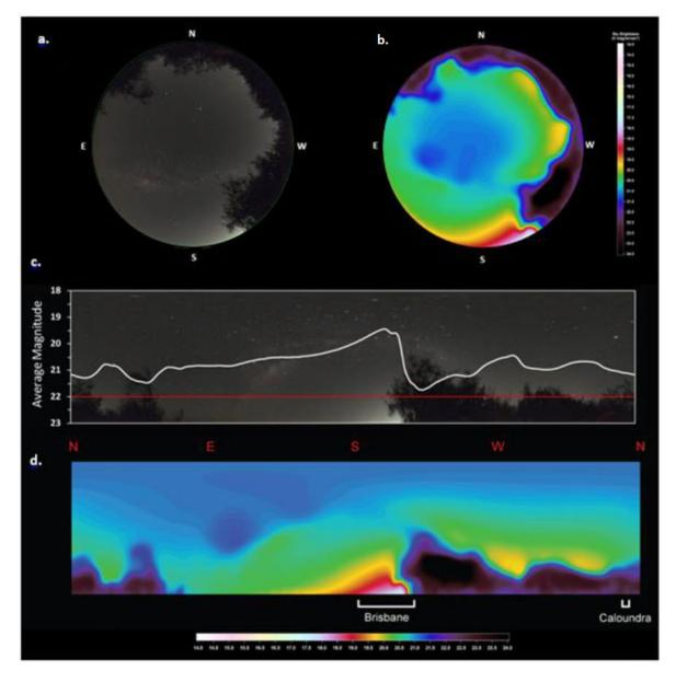
Figure 5: Sky42<sup>™</sup> output showing; a. typical image of night-sky captured by Sky42<sup>™</sup>; b. example isophote map of light levels across the visible spectrum (see Table 3 for interpretation); c. bearing (°) and average magnitude of measured light; d. isophote image of night sky shown 0° - 359° Notes: X axis: bearing from 0° - 359°, Y axis: average magnitude (V mag/arcsec<sup>2</sup>). Red line: target magnitude, representative of a rural dark sky i.e. unaltered night sky horizon.
