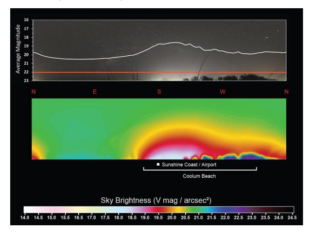
**Figure 32: Bearing (°) and average magnitude in cloudy sky conditions, measured in June 2017 from Coolum beach north, Sunshine Coast.** X axis: bearing from 0° - 359°, Y axis: average magnitude (V mag/arcsec<sup>2</sup>). Red bar: 'ideal' or 'target' light level - average magnitude 22 or less.
