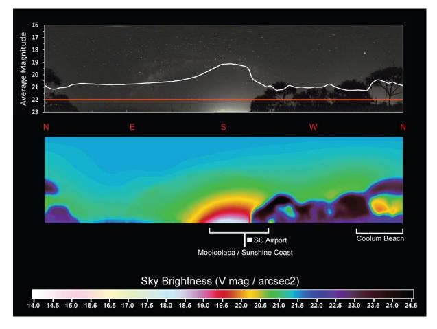
**Figure 30: Bearing (°) and average magnitude in cloudy sky conditions, measured in June 2017 from Yaroomba beach north, Sunshine Coast.** X axis: bearing from 0° - 359°, Y axis: average magnitude (V mag/arcsec<sup>2</sup>). Red bar: 'ideal' or 'target' light level - average magnitude 22 or less.
