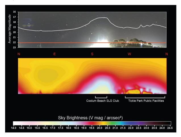
**Figure 31**: Bearing (°) and average magnitude in cloudy sky conditions, measured in June 2017 from Coolum Beach south, Sunshine Coast. X axis: bearing from 0° - 359°, Y axis: average magnitude (V mag/arcsec<sup>2</sup>). Red bar: 'ideal' or 'target' light level - average magnitude 22 or less.
