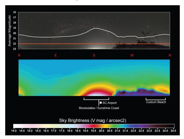
**Figure 29: Bearing (°) and average magnitude in cloudy sky conditions, measured in June 2017 from Yaroomba beach south, Sunshine Coast.** X axis: bearing from 0° - 359°, Y axis: average magnitude (V mag/arcsec<sup>2</sup>). Red bar: 'ideal' or 'target' light level - average magnitude 22 or less.
