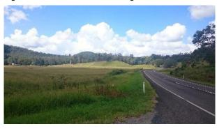
The eastern access is a secondary access to the site and is only used during major events by competitors. Sight lines to/ from this access are severely restricted in both directions by vertical and/ or horizontal curves. The poor sight lines at this location has led to the requirement for a TMP to be implemented at this access during the main events.
