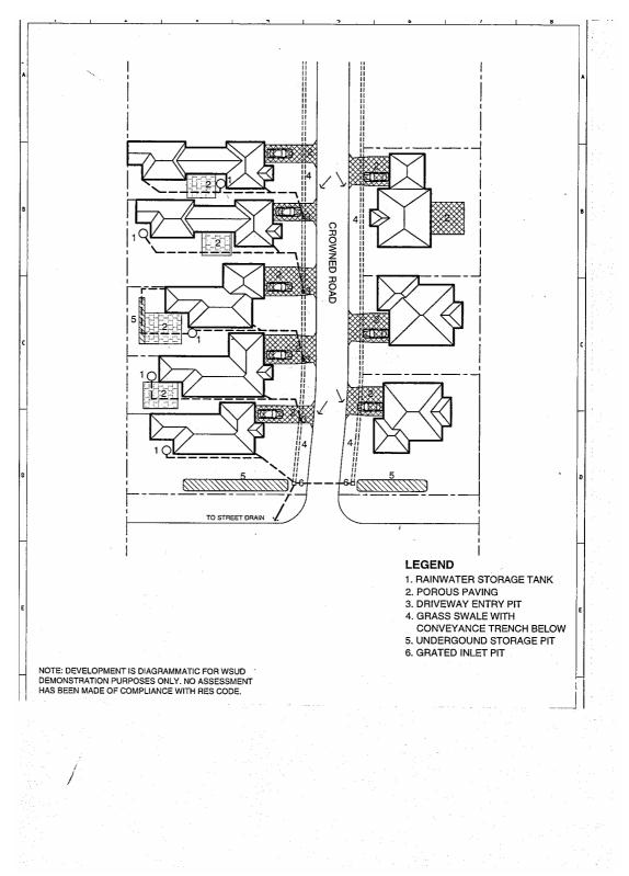
Figure 5.5 – Typical Detached Unit or Integrated Housing Development (Lot size between 350m<sup>2</sup> and 450m<sup>2</sup>).
