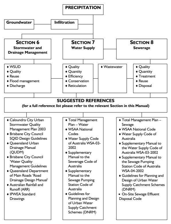
Figure 5.2 – Application of Total Water Cycle Management
