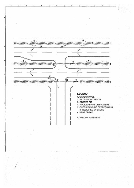
Figure 5.8 – Roadway Installation
