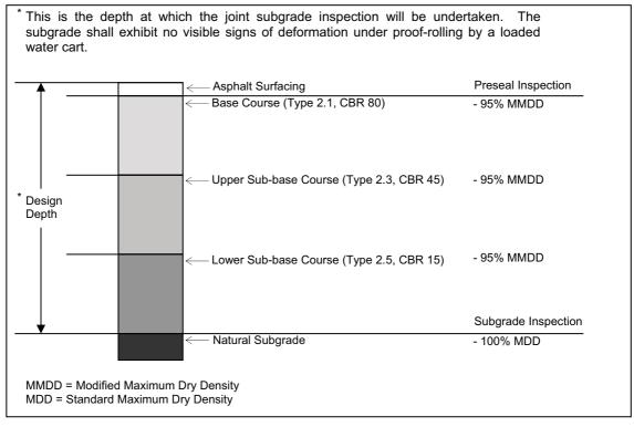
Figure 3.2 – Schematic Pavement Cross Section
