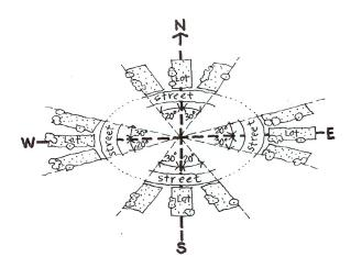
Figure 4.2.3(a) – Desirable Orientation Range for Street and Lot Layout
