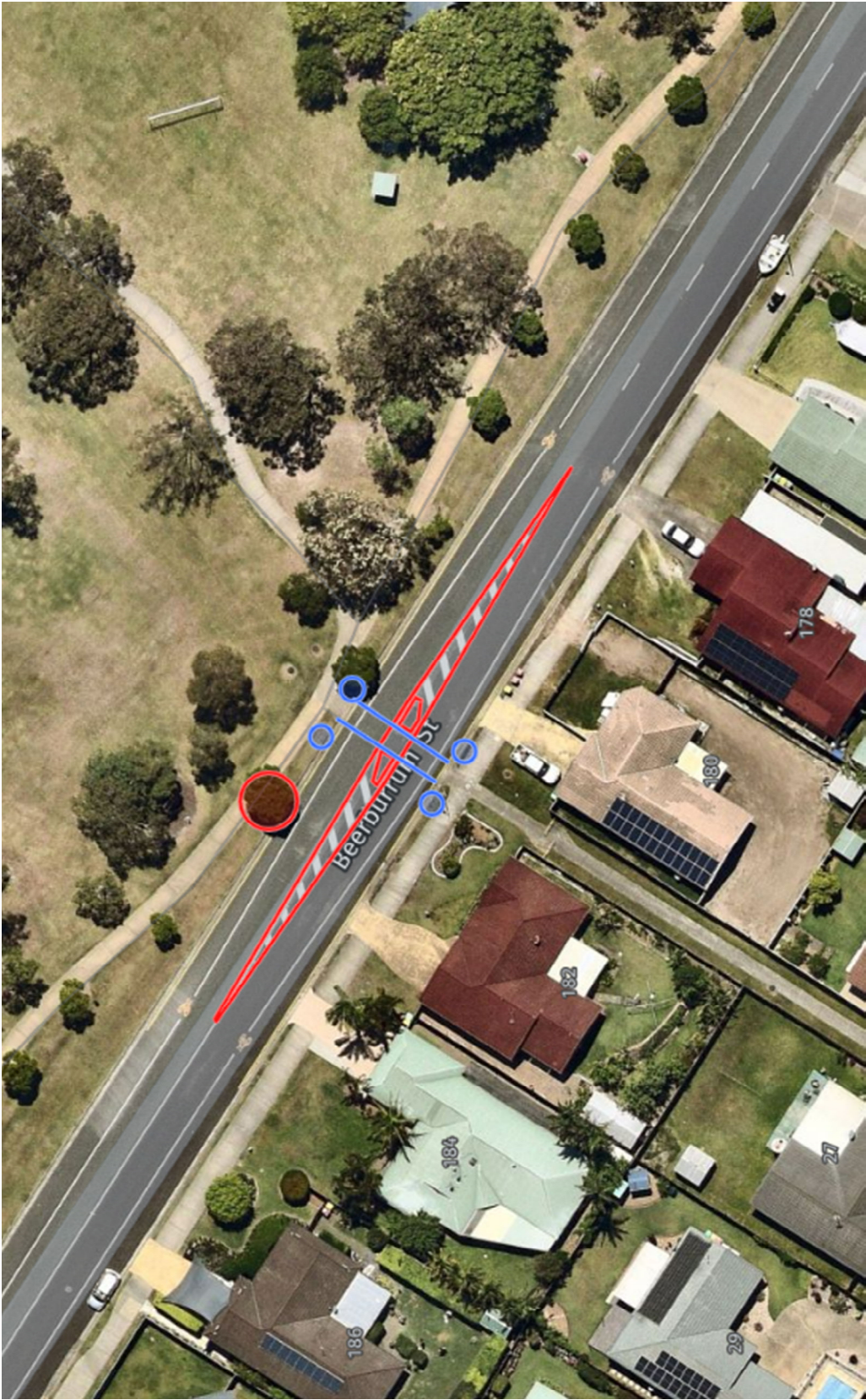
Figure 1: New pedestrian crossing location Removal of line marking, refuge isles and tree. Placement of new traffic signals and pedestrian crossing
