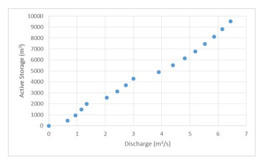
Figure 11 Example Storage-Discharge relationship
