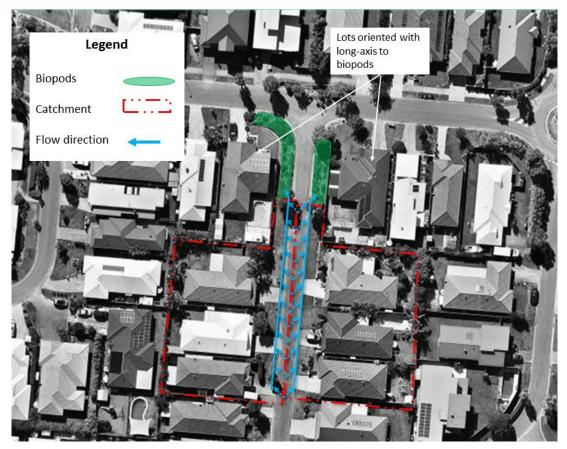
Figure 5 Biopod Locations for Centrally Crowned Access Street
