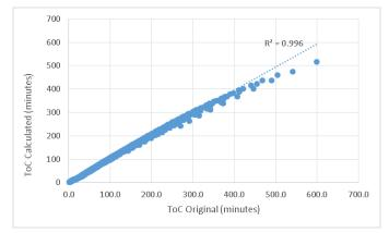
Figure 11 ToC estimates: Formula Estimates vs Model Derived
