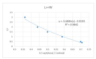
Figure 13 CF equation for catchments where Length ≥ Width
