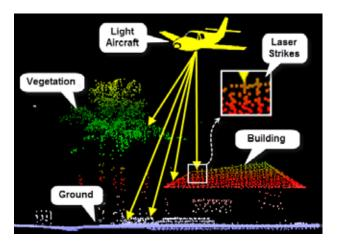
Figure 1: Profile view of LiDAR mapping technique
