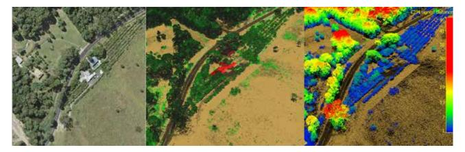
Figure 3: pictured from left to right: Aerial Orthophoto of a semi-rural area containing open grassed areas, regularly spaced fruit trees, a rural road and some natural vegetation; (MIDDLE) an oblique view of a colourised *LiDAR* data point cloud showing tree vegetation in green, buildings in red, and the ground in brown and black; and (RIGHT) the same *LiDAR* point cloud coloured according to height above ground in a range of colours from blue (shortest) through green, yellow and red (tallest).
