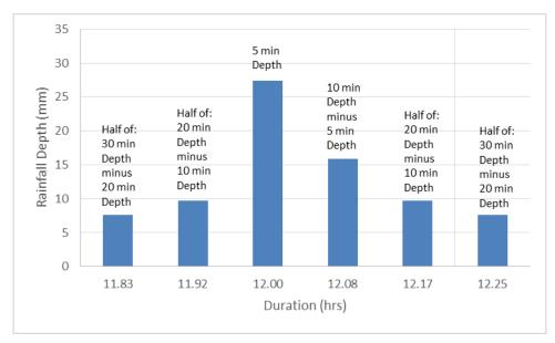
Figure 13 Demonstrating the calculation of a Duration Independent Storm Temporal Pattern
