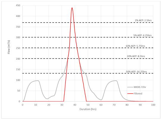
Figure 9 MIDIS Hydrograph Filtering
