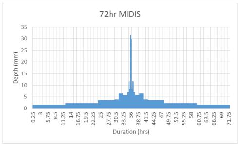
The peak from a hydrograph generated using a MIDIS temporal pattern was observed to show good agreement with critical duration analysis using ensemble and MIS methodologies.
