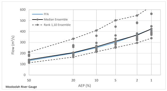
Figure 1 Comparison of the Mooloolah River FFA with Design Results derived using Ensemble Patterns
