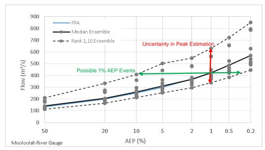
Figure 2 Comparison of the Mooloolah River FFA with Design Results derived using Ensemble Patterns
