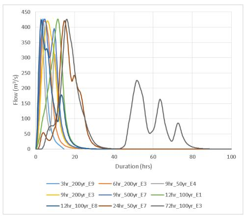
Figure 3 1% AEP Discharge Hydrographs from Ensemble Hydrographs
