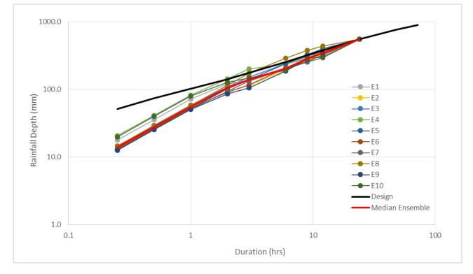
4. Calculate the MIS temporal pattern using the methodology of a Duration Independent Storm (DIS) as documented in Appendix A. Use the calculated median intensities instead of design intensities.
