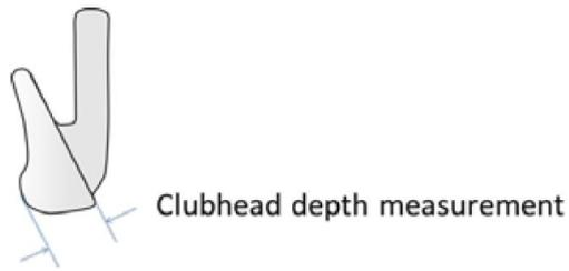
Figure 2 Definition of the clubhead depth for Section 3.c(i).
