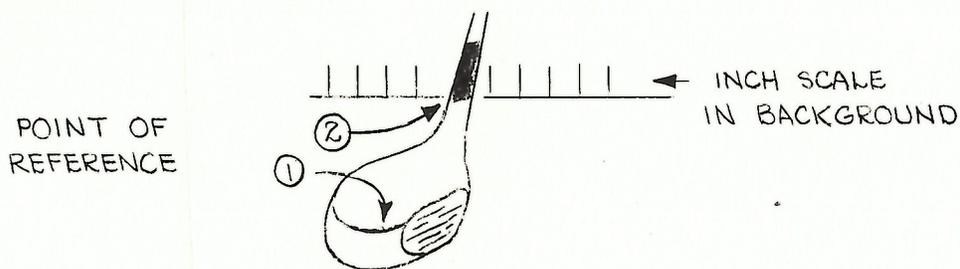
This was the only well-defined light mark on the otherwise dark clubhead. We repeated measurements of this point on the original photographs using a travelling microscope. (The original measurements were made with a fine scale.) These microscopic measurements tallied with the original ones.
