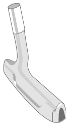
(a) Putter with hole extending from toe to heel (conforming).
