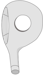
Wood head with hole from crown to sole (non-conforming).
