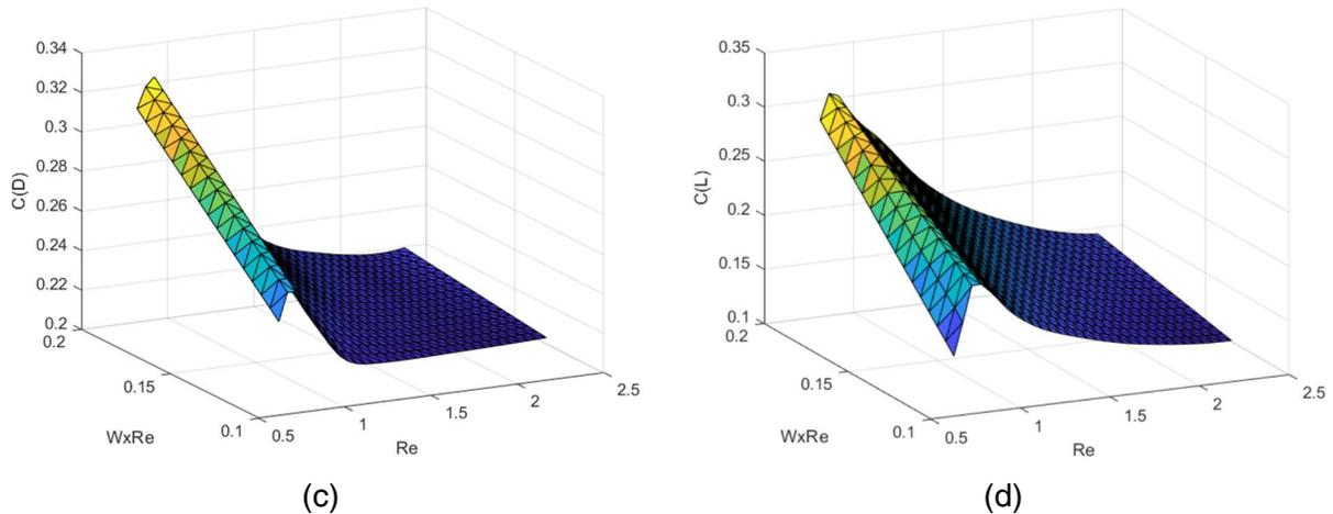
Figure 1: Graphical depiction of lift and drag coefficients for a high-performance TOUR-type golf ball (a, b) and a ball with high Reynolds number sensitivity (c, d) as functions of Reynolds number and nondimensional spin (see Table 5, ball type “D”).
