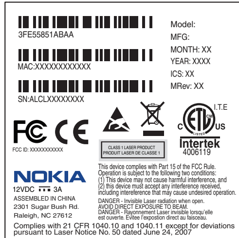
Figure 4-6 Sample laser product safety label on the ONT equipment
