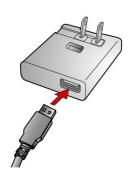
2. Connect the micro USB connector to the micro USB port at the bottom of the device.
