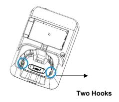
Use your thumb to lift up and take out the detachable part. Once it is unhooked, you can lift it up from both sides.
