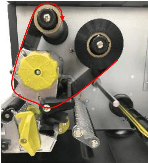
4. Thread ribbon below the ribbon guide bar through ribbon sensor slot as the loading path printed on the printer.
