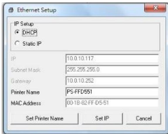
The default IP address is obtained by DHCP. To change the setting to static IP address, click “Static IP” radio button then enter the IP address, subnet mask and gateway. Click “Set IP” to take effect the settings.
