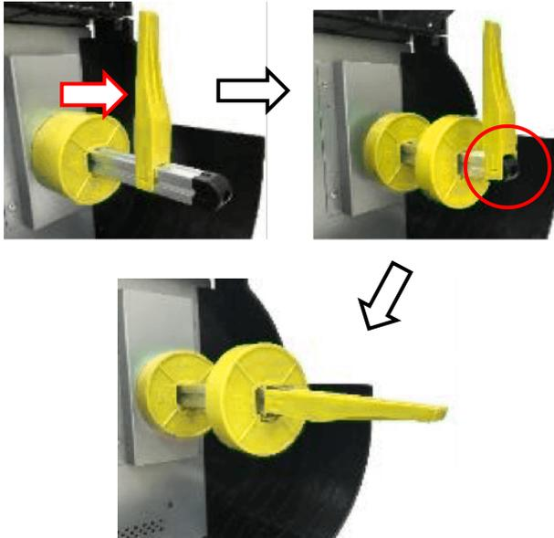
2. Move the label roll guard horizontally to the end of label spindle, then flip down the label roll guard.
