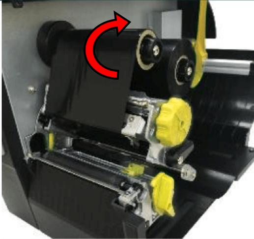
6. Wind the ribbon rewind spindle counterclockwise roughly 3~5 circles until the ribbon is smooth, properly stretched and wrinkle-free.
