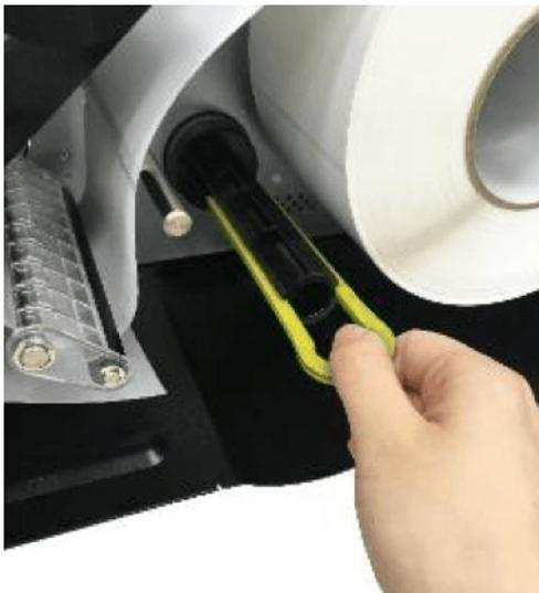
7. Pull out the media rewind spindle securing clip. Wind the media on the spindle until the liner stretched properly.
