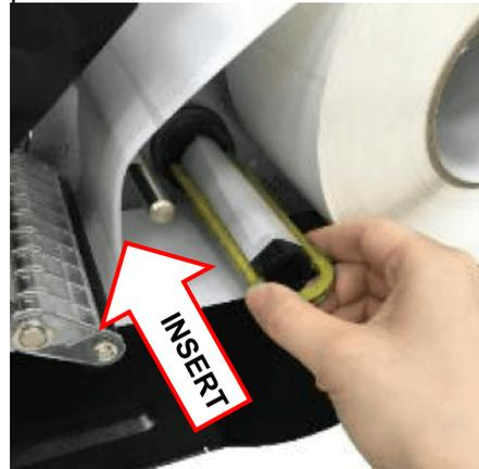
Note: The media rewind spindle can also install paper roll to wind the media on media rewind spindle.
