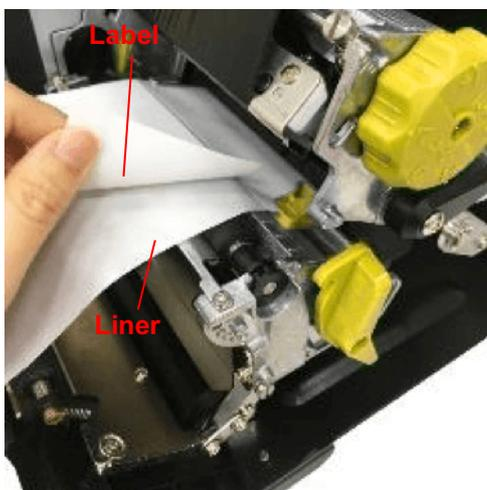
4. Open print head release lever, pull approximately 650 mm of the label through the front of the printer.
