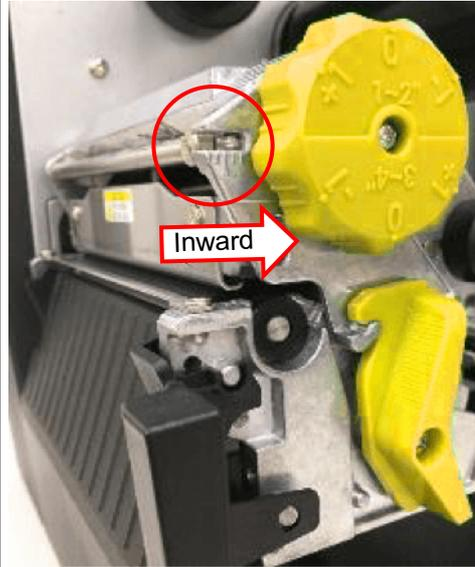
2. If the ribbon tension adjustment knob has positioned on the level of innermost side but didn't improve the ribbon wrinkle, please switch the print head pressure adjustment knob per 1 level and print the label again to check if the wrinkle is gone.
