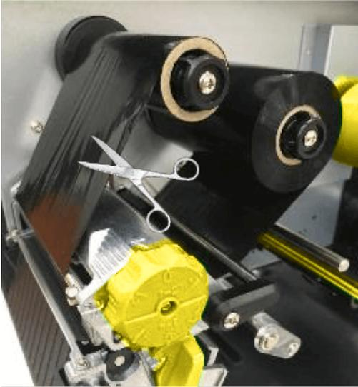
1. Break the ribbon between ribbon guide plate and the ribbon rewind spindle.
