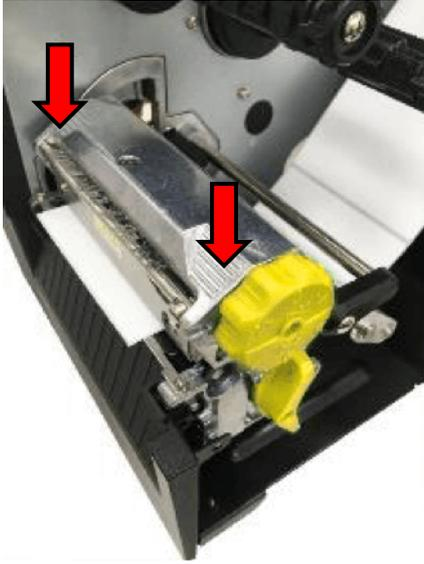
7. Close the print head mechanism on both sides and make sure the latches are engaged securely.
