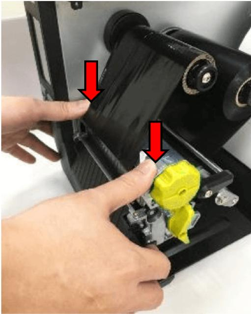
7. Close the print head mechanism by pushing down the both sides of the print head release lever.
