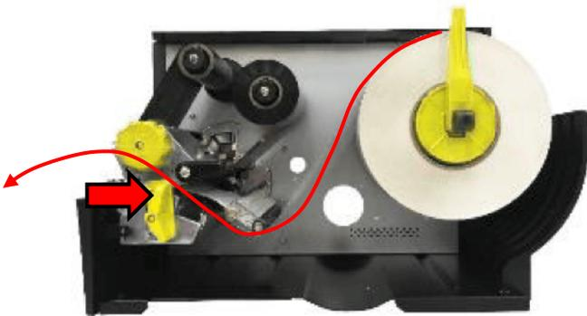
4. Push the print head release lever and install the label through the damper, media sensor, and label guide to install the media.
