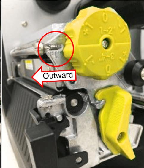
2. If the ribbon tension adjustment knob has positioned on the level of outermost side but didn't improve the ribbon wrinkle, please switch the print head pressure adjustment knob per 1 level and print the label again to check if the wrinkle is gone.
