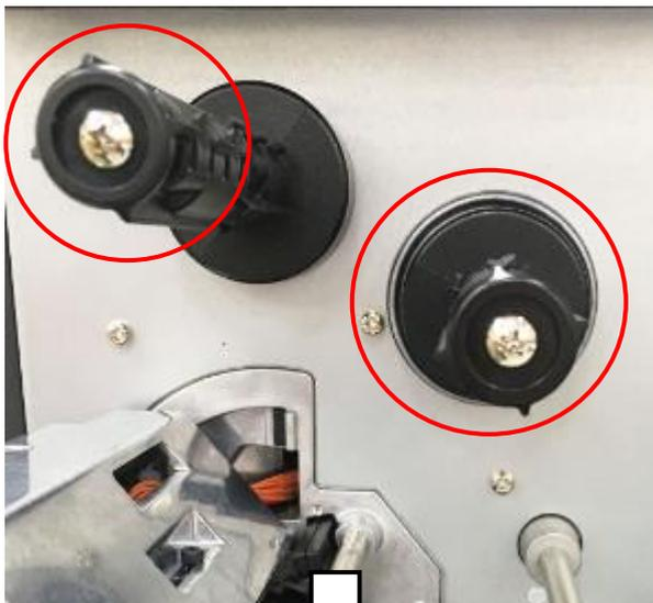
2. Install the ribbon onto ribbon supply spindle and install paper core onto ribbon rewind spindle.
