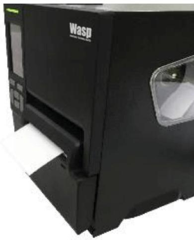
5. Close the print head mechanism and press the FEED button to test.
