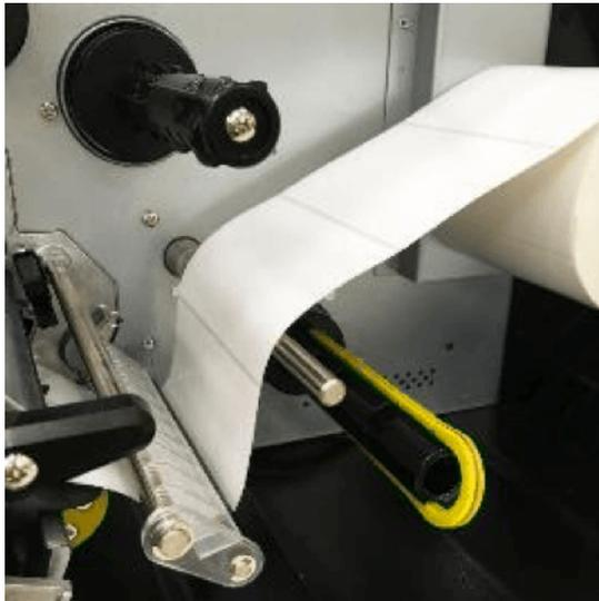
3. Using the front display panel to do the calibration first and set the printer mode to peeler mode.
