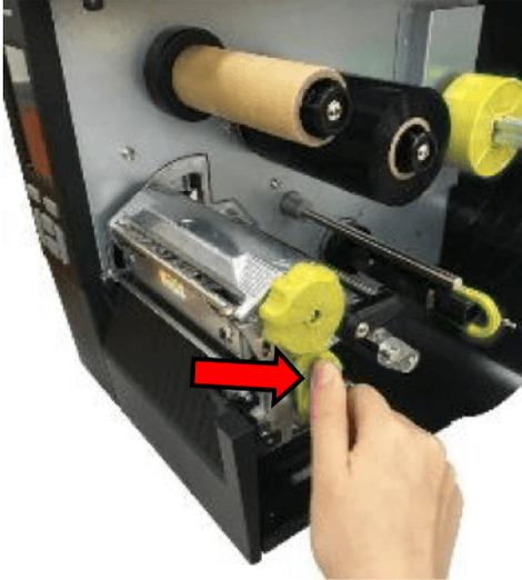
3. Push the Print head release lever to open print head mechanism.
