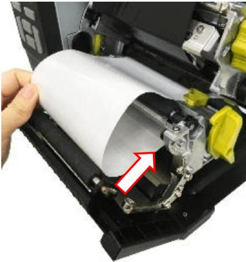
6. Feed the leading edge of liner through the peel-off module slot as indicated.
