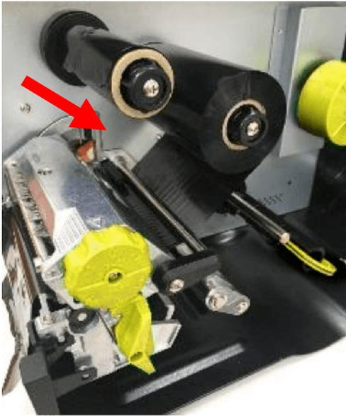
2. Slide the ribbon off to release the ribbon on the ribbon rewind spindle.
