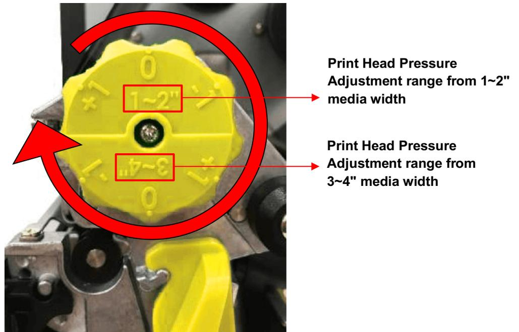
The print head pressure adjustment knob has 6 levels of adjustment for 1~2" and 3~4" media widths. Because the printer's paper alignment is to the left side of mechanism, different media widths require the different pressure to print the label correctly. Therefore, it may require adjusting pressure to get the best print quality.
