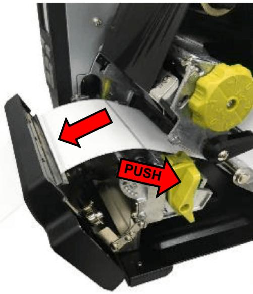
4. Push the Print head release lever to open print head mechanism. Lead the media through the cutter paper opening.
