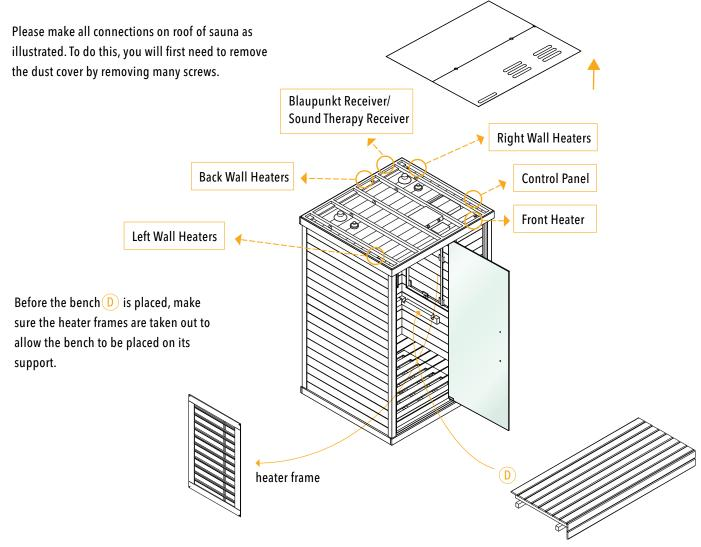
NOTE: The right wall of the sauna includes wire connections underneath which will lead into the floor panel (see illustration 7.2 below).
