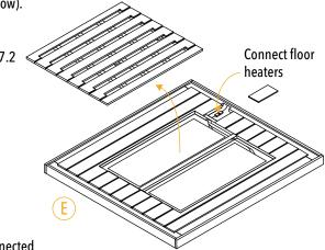
The floor heaters will need to be connected to the right wall wires. The diagram above shows where the connection is made. You will need to remove the floor grate and a small hatch covering the harness.
