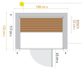
POWER 240V, 2251 watts. Dedicated 15A circuit and 15A power socket protected by a 16A RCBO installed in the meter box. Minimum 2.5mm cable required for circuit; 2.5m cord exits from back left side of roof.
