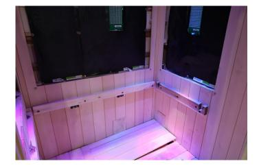
To remove the bench, unmount the heater frames from the surrounding walls. Reach underneath, with your palms upward, and the bench will lift straight up from the supports mounted to the walls (for Discover and Empower cabins, you only need to remove the back-wall bench sections). You can then rotate the detached bench vertically and walk it backwards out of the sauna.
