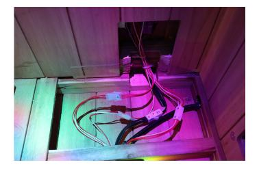
Disconnect the G4 power connector from the F7 power cables. Disconnect the G28 sensor line from the corresponding F8 connector. You'll find a connector that is covered with black tape (red/ white wires) and zip-tied with a screw anchoring it to the base. Unscrew the anchored zip tie.
