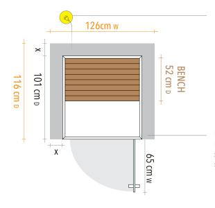
POWER 240V, 1673 watts. Dedicated 10A circuit and 10A power socket protected by a 10A RCBO installed in the meter box. Minimum 2.5mm cable required for circuit; 2.5m cord exits from back left side of roof.
