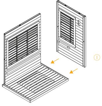
If you have not yet done so, the floor heaters will need to be connected to the right wall wires. The diagram to the left shows where the connection is made. You will need to remove the floor grate and a small hatch covering the harness.
