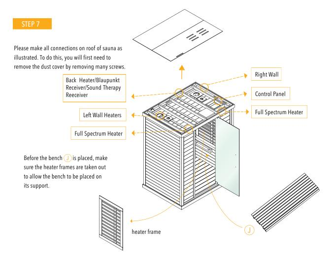
With the bench installed, the heater panel frames can be inserted back into their respectable walls.
