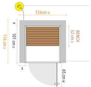
**POWER REQUIREMENTS** 220–240V, 1707 watts. Maximum Amperage 10A. Sunlighten recommends all new installations adhere to AS3000 and a circuit that is RCD protected, along with a readily accessible switch.
