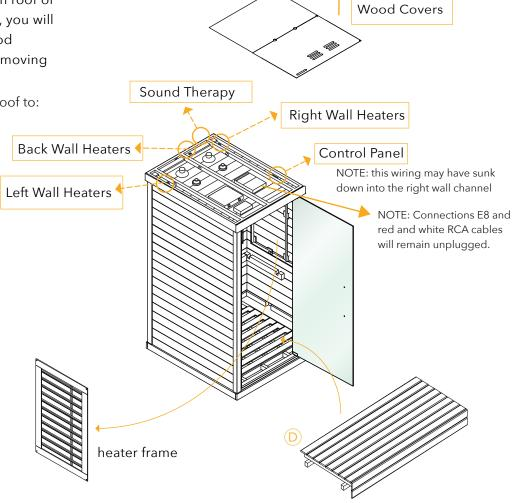
The floor heaters will need to be connected to the right wall wires. The diagram to the right shows where the connection is made. You will need to remove the floor grate and a small hatch covering the harness (see illustration 7.2).
