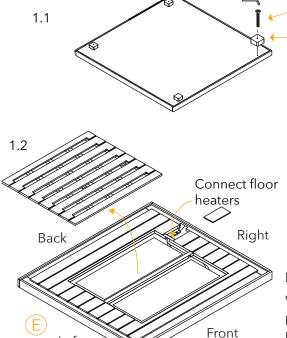
NOTE: Ensure the side with the removable wood panel is on the right side before step 2.
