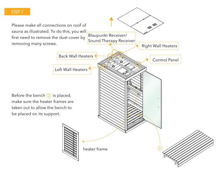
NOTE: The right wall of the sauna includes wire connections underneath which will lead into the floor panel (see illustration 7.2 on the right).
