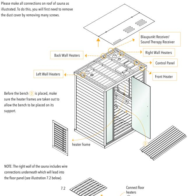
The floor heaters will need to be connected to the right wall wires. The diagram to the right shows where the connection is made. You will need to remove the floor grate and a small hatch covering the harness.
