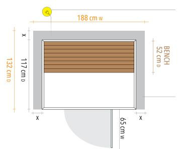
POWER 240V, 2251 watts. Dedicated 15A circuit and 15A power socket protected by a 16A RCBO installed in the meter box. Minimum 2.5mm cable required for circuit; 2.5m cord exits from back left side of roof.
