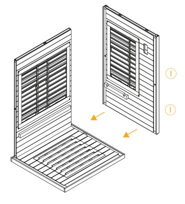
If you have not yet done so, the floor heaters will need to be connected to the right wall wires. The diagram to the left shows where the connection is made. You will need to remove the floor grate and a small hatch covering the harness.
