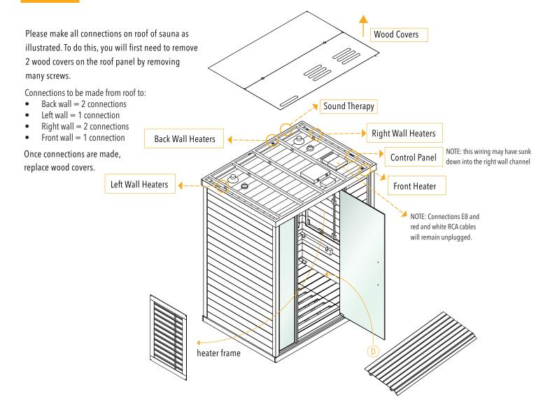
The floor heaters will need to be connected to the right wall wires. The diagram to the right shows where the connection is made. You will need to remove the floor grate and a small hatch covering the harness (see illustration 7.2).
