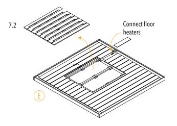
The floor heaters will need to be connected to the right wall wires. The diagram to the left shows where the connection is made. You will need to remove the floor grate and a small hatch covering the harness.
