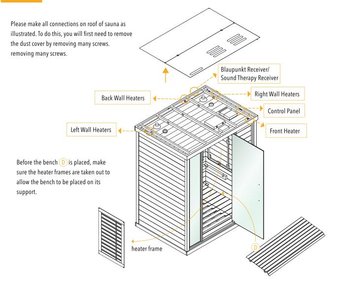
NOTE: The right wall of the sauna includes wire connections underneath which will lead into the floor panel (see illustration 7.2 below).
