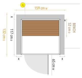
POWER 240V, 2251 watts. Dedicated 15A circuit and 15A power socket protected by a 16A RCBO installed in the meter box. Minimum 2.5mm cable required for circuit; 2.5m cord exits from back left side of roof.
