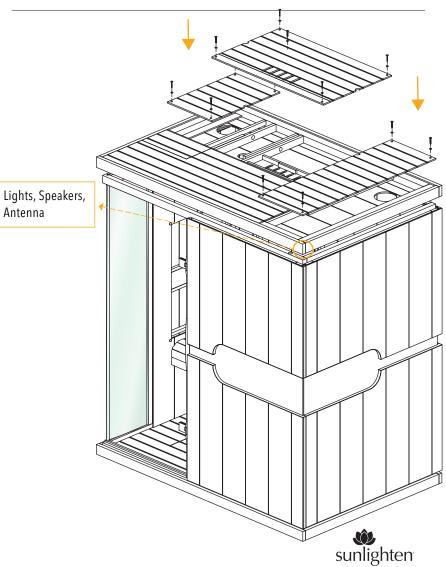
The dust cover should be replaced to protect the lights and speakers from dust and other floating residue. Place the heater frames in their respective locations if you have not yet done so. As mentioned in STEP 5, there are four connections to be made in each bottom section of the walls. If you have not yet done, so consult with the diagram at the bottom of this page.
