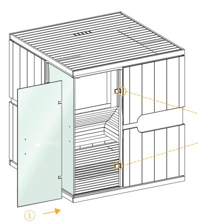
The gaskets, bolts and washers (1, 2) and (3) will come with the handles. The washers need to be inserted into the door holes first before the gaskets go on and eventually the bolts. The rough side of the gaskets must be facing the glass door. Be sure to have a second person hold the handle in place while the other inserts the bolt.
