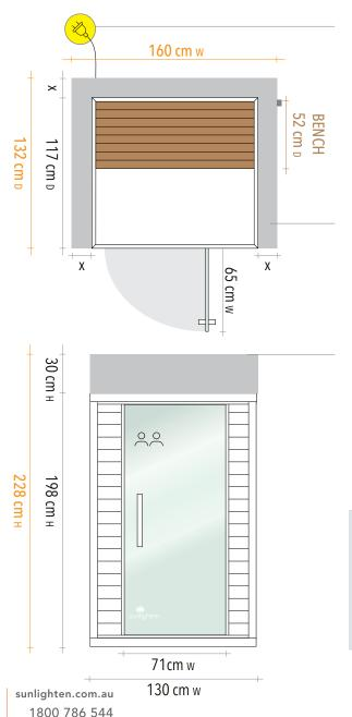
POWER REQUIREMENTS 220-240V, 2231 watts. Maximum Amperage 11A. Sunlighten recommends all new installations adhere to AS3000 and a circuit that is RCD protected, along with a readily accessible switch.
