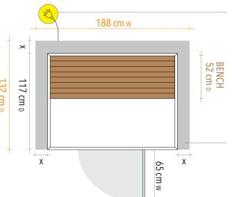
**POWER REQUIREMENTS** 220–240V, 2371 watts. Maximum Amperage 15A. Sunlighten recommends all new installations adhere to AS3000 and a circuit that is RCD protected, along with a readily accessible switch.
