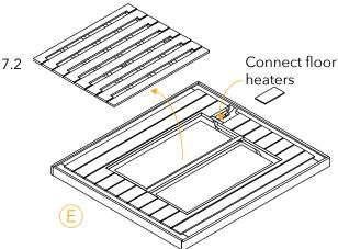
The floor heaters will need to be connected to the right wall wires. The diagram above shows where the connection is made. You will need to remove the floor grate and a small hatch covering the harness.
