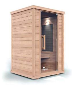
POWER 240V, 2251 watts. Dedicated 15A circuit and 15A power socket protected by a 16A RCBO installed in the meter box. Minimum 2.5mm cable required for circuit; 3m cord exits from back left side of roof.
